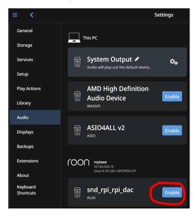
3. After enabling the device, select the gear icon and then hit "Device Setup".
