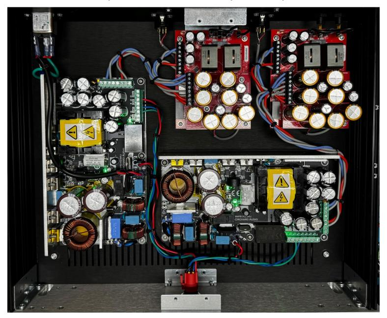
Fully Assembled Dual Mono Amplifier Example
