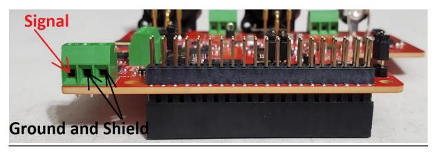
The S/PDIF input has an automatic switch over that routes audio from the S/PDIF connection when there is a valid signal. When no valid signal is available on the S/PDIF interface the device defaults to accepting data from Rpi or Tinker Board.
