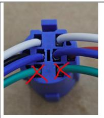
NOTE: On some of the harnesses wire colors are different. The Yellow wires are not used instead of green.
